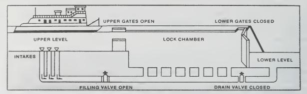
The lower lock gates are closed; the drain value is closed; the filling value is open; the lock has filled to the level of the upriver pool; and the upper lock gates have been opened to allow the towboat to enter the lock
