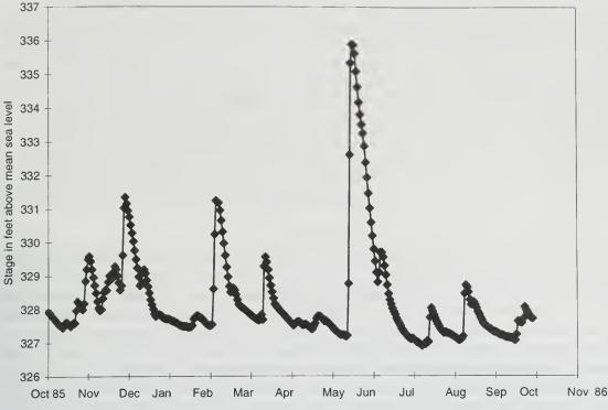
Figure 19 Water-level elevation in Buttonland Swamp recorded at the IL 137 bridge by the Illinois State Water Survey (modified from Demissie et al. 1990b).
