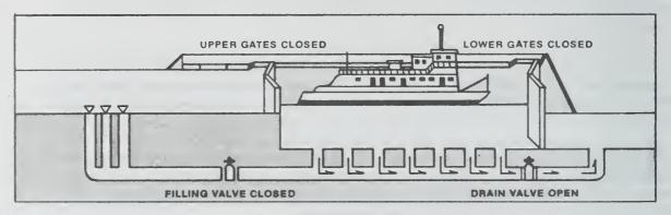
Now the towboat is in the lock; the upper lock gates have been closed; the filling valve is closed; the drain valve is open, allowing water to drain into the downriver pool. The towboat is lowered as the water level lowers
