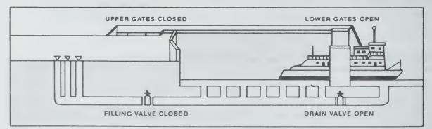
The water in the lock has here reached the level of the downriver pool. The lower lock gates have been opened and the towboat is leaving the lock to proceed on its way downriver
