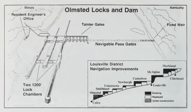
Figure 14 Artist's rendition of the New Locks and Dam at Olmsted (modified from U.S. Army Corps of Engineers).
