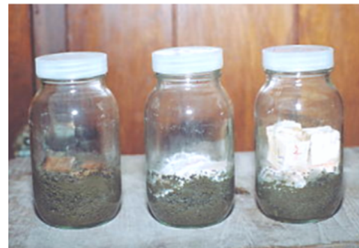
g. Accelerated laboratory test for natural decay resistance in poplar wood
