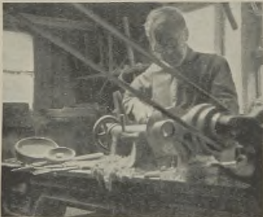
Electrically driven hand-turning lathes at Davies & Sons' woodworking factory at Abercethy
