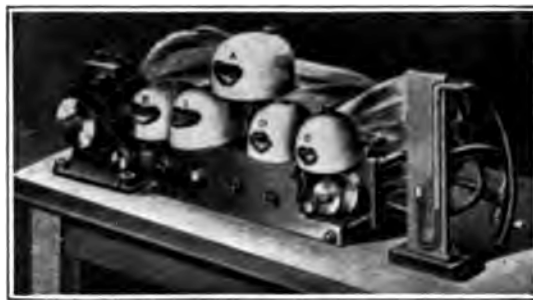
Figure 3. Apparatus for imitating vowels, developed by Marage in Paris, consisting of artificial larynxes, mouths, and nasal cavities driven by a bellows and motor as lungs. Reprinted from Dayton C. Miller, The Science of Musical Sounds (New York: Macmillan Co., 1916), 244.
