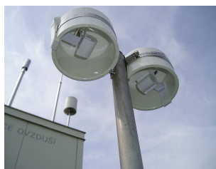
Figure 2. Collocated measurement of Ogawa sampler and real-time monitor
